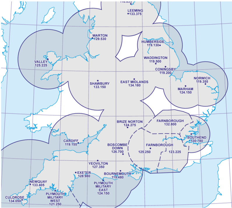
Extract from, and full page available from UK AIP ENR 6-10 LARS showing intended coverage.
